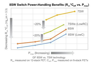
8SW delivers a high  $f_t/f_{max}$ , supporting diversity receive and main antenna path LNA applications for today's 4G and future sub-6 GHz 5G operating frequencies.
